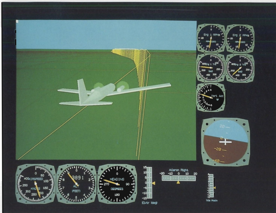
Using an HP 9000 TurboSRX Series 835 computer and an HP 98748A high-resolution monitor, CASB scientists can simulate the September 1988 flight of the Hawker-Siddeley 748.
